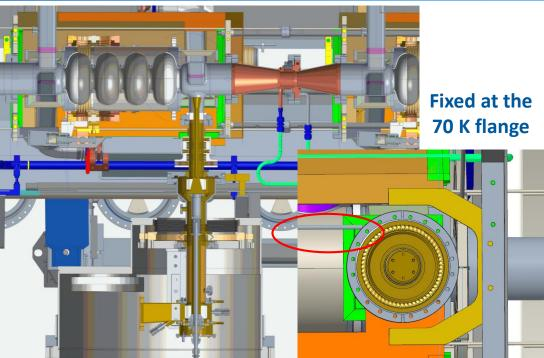
The coupler is a fixed point within the module. → during cooldown, displacement of the coupler tip can be expected.
