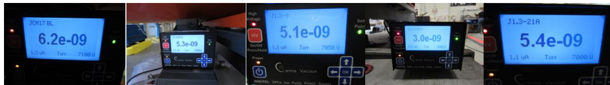
RT BL vacuum on different CMs during wFPC installation
