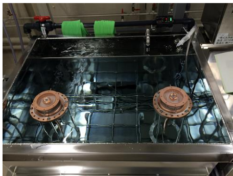
Ultrasonic cleaning with ultrapure water
