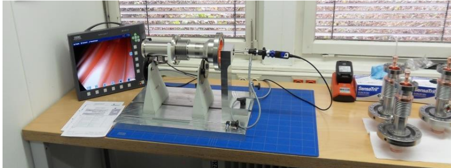
Visual inspection of the copper plating at RI
