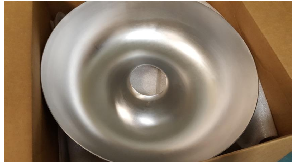
Post-BCP salted water soak
