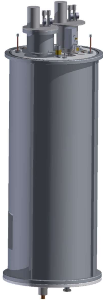
Vacuum vessel w/ magnetic and 80 K shields
