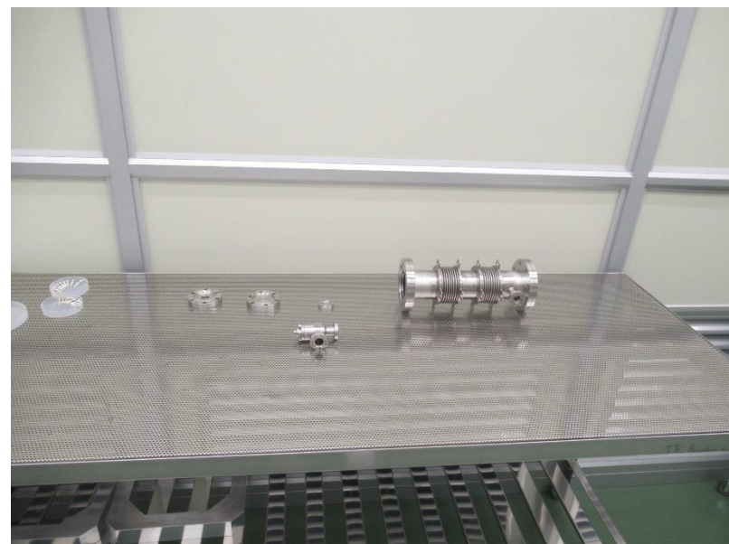
Wash the bellows by ultra-pure water and dried in class 10
