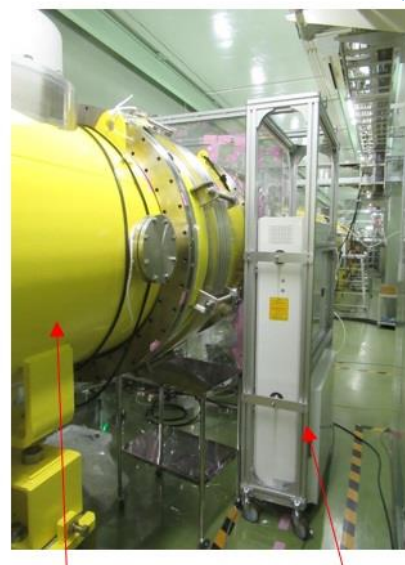
Slow pumping system KOACH (A) Changing room STF-2 cryomodule KOACH (B)
