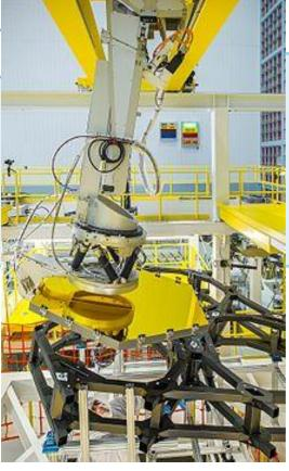
Robotic arm installing mirror segments for the James Webb Space Telescope - NASA
