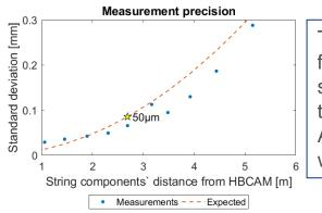
The measurement uncertainty for each component in the string assembly depends from the distance to the camera. Acquired data are matching with the expected precision.
