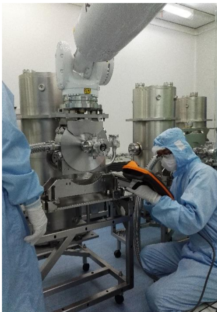
Solenoid assembly and fixing on the bracket
