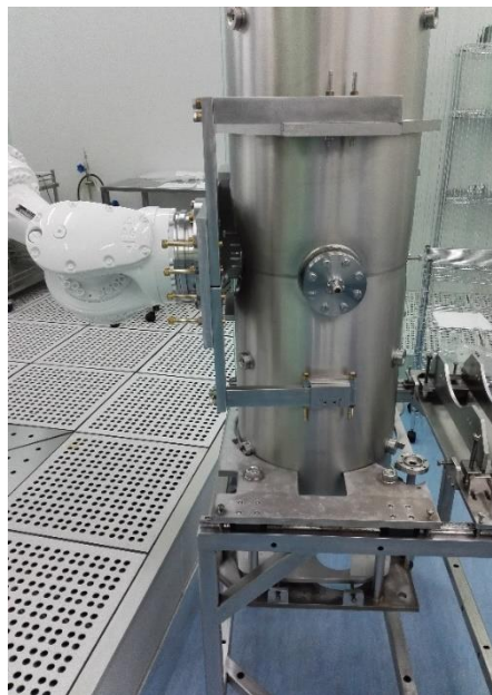
Cavities moving and fixing on the bracket
