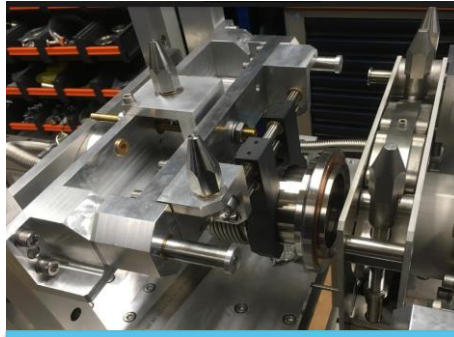
VAX Module interconnection – chain clamp DN100 in b.112
