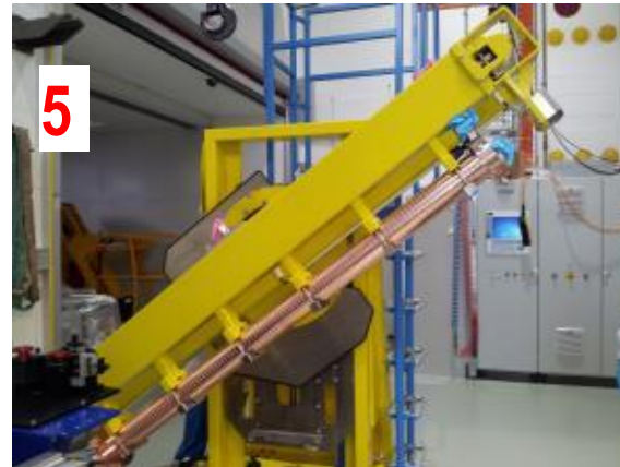
Structure reversed to horizontal position on a temporary girder
