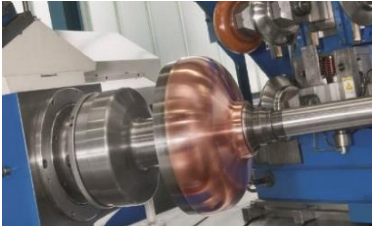
Left: Half-Cell by Spinning + internal machining (HEGGLI, CH),
