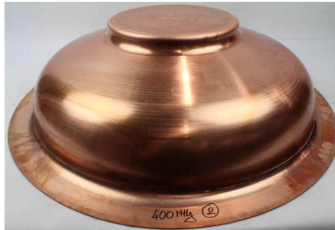
Left: Half-Cell by Spinning + internal machining (HEGGLI, CH),
