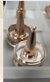
Four high power HOM couplers fabricated and low power tested with cavity. Three will mount on the 2-cell cavities. Vertical test soon with the cavity to verify the notch properties. High power test (1 kW) at RT and 2 K planned with special rigid coaxial line.
