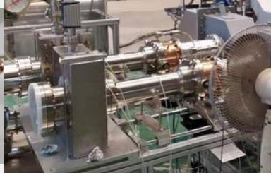
High power test of one 650 MHz fixed coupling input coupler reached 150 kW SW (corresponding to 400 kW TW at the window). Another coupler's window broke due to excess ceramic heating. New window and two variable couplers in fabrication.
