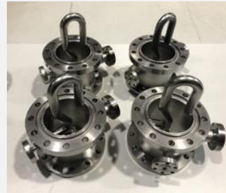
Four high power HOM couplers fabricated and low power tested with cavity. Three will mount on the 2-cell cavities. Vertical test soon with the cavity to verify the notch properties. High power test (1 kW) at RT and 2 K planned with special rigid coaxial line.
