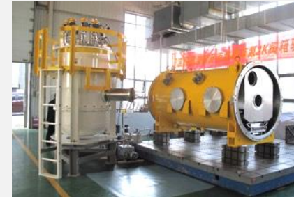
Cryomodule and valve box for two 650 MHz 2-cell cavities etc. Module assembly and beam test at PAPS in 2020.
