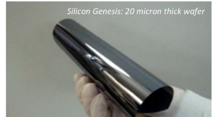
Ultra-thin chip (<50 μm): flexible with good stability
