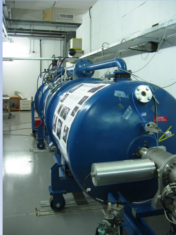
Accelerator tank filled with 3 bar SF 6
