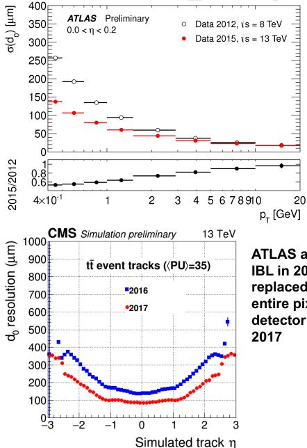
Adding a layer at smaller radius (red points) improves impact parameter resolution
