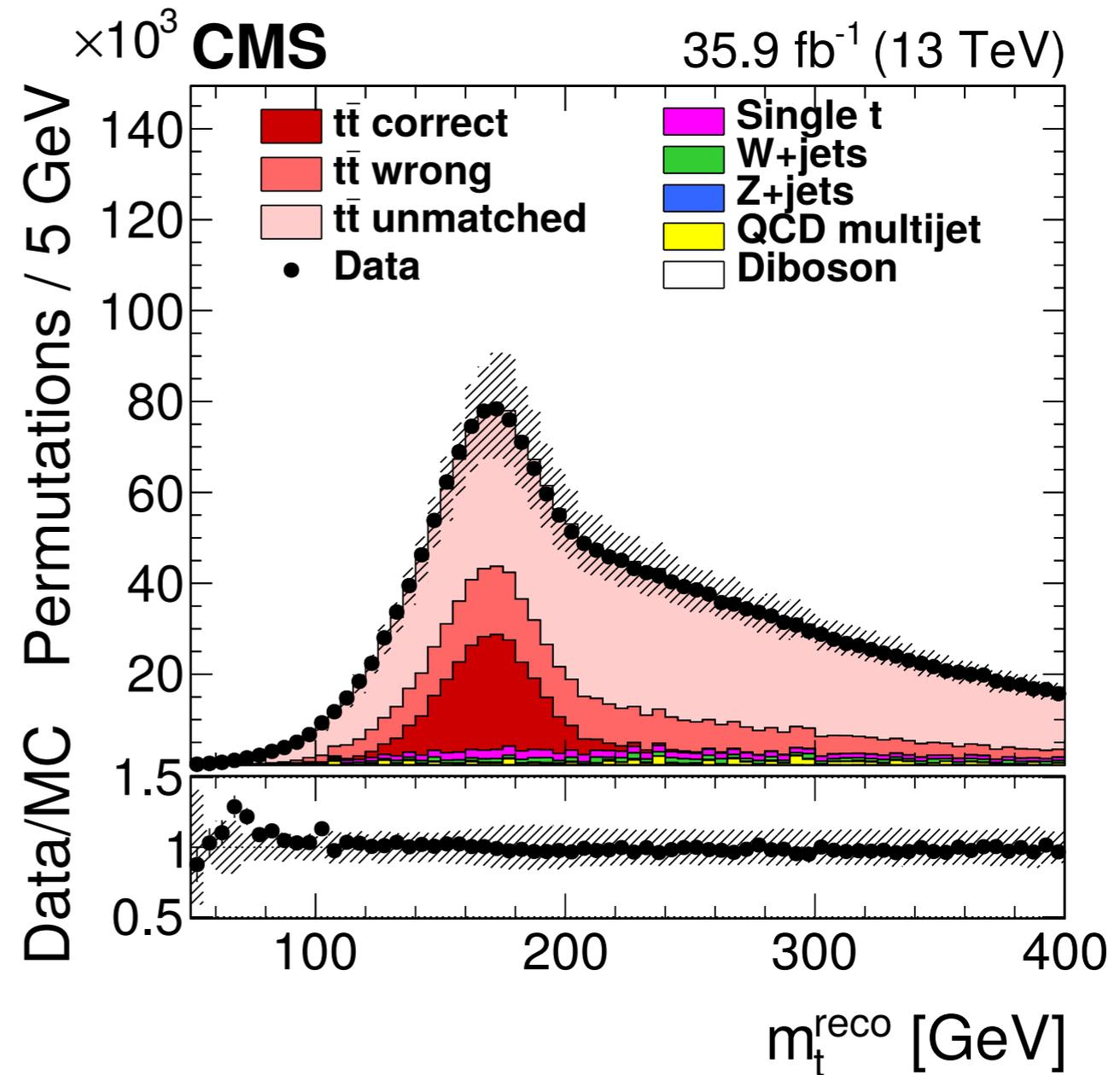
Use templates to fit  $m_{jjb}$ , constrain jet energy with fit to  $m_{jj}$
