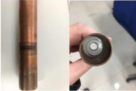
CrZrCu ( \phi 24 \times 1 ) pipe welding test
