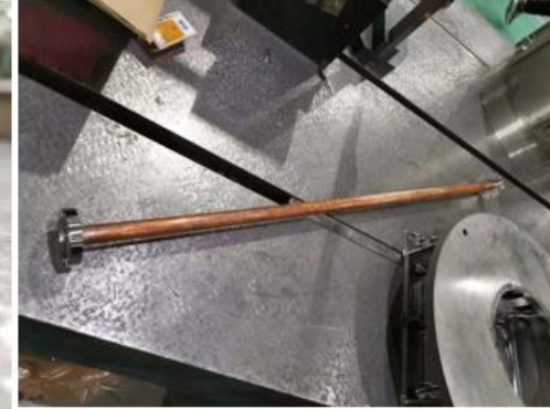
CrZrCu ( \phi 24 \times 1 ) pipe and Stainless Steel flange welding test
