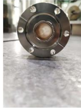
CrZrCu ( \phi 24 \times 1 ) pipe and Stainless Steel flange welding test
