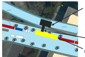
Laser electronics in side tunnel Used for electron transfer during LEP time Optical transport line on the ceiling Cavity
