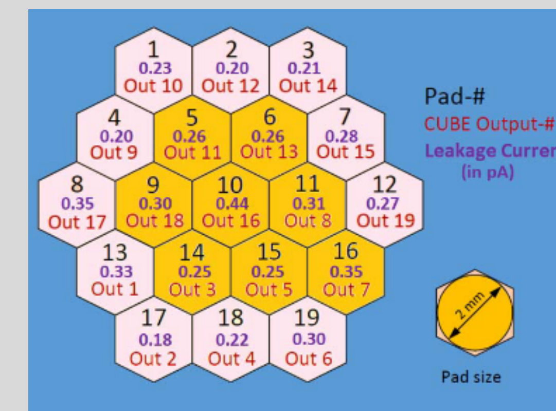
Fig. 1 : Schematic of the current DLS-SOLEIL prototype. The proposed demonstrator is composed of 19 hexagonal pixels of 2 mm inner diameter.
