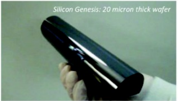
Ultra-thin chip (<50 um): flexible with good stability
