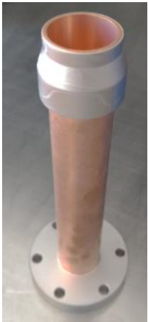
Pumping out pipe
