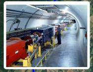
Maximum Beam Momentum:  $Z \times 450$  GeV/c, accelerates p,  $\bar{p}$ , O, S, Ar, Pb..
