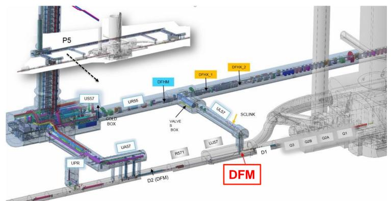
Interface between SC Link and D2. It provides the powering of the HL-LHC Matching Sections (D2 and its correctors)
