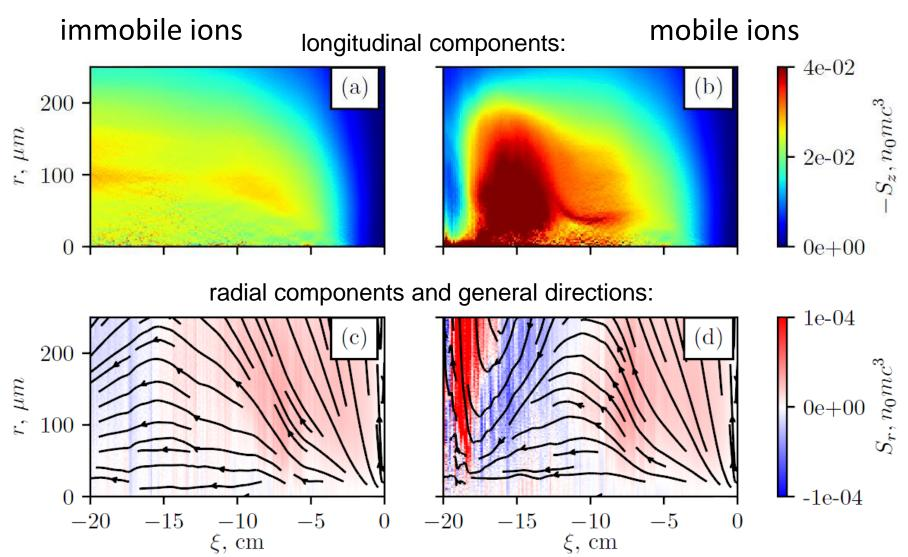
Ion non-uniformity causes concentration of the wave energy near the axis
