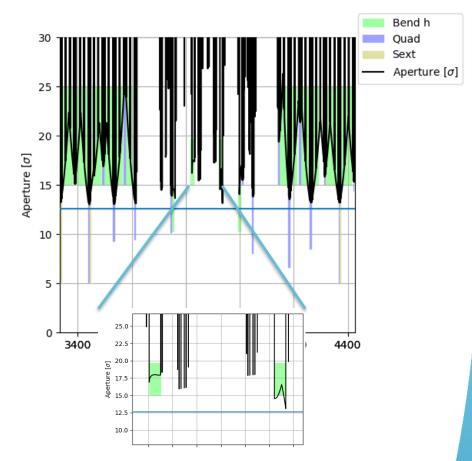
Aperture margin for e-lens available, to be evaluate with detailed drawings
