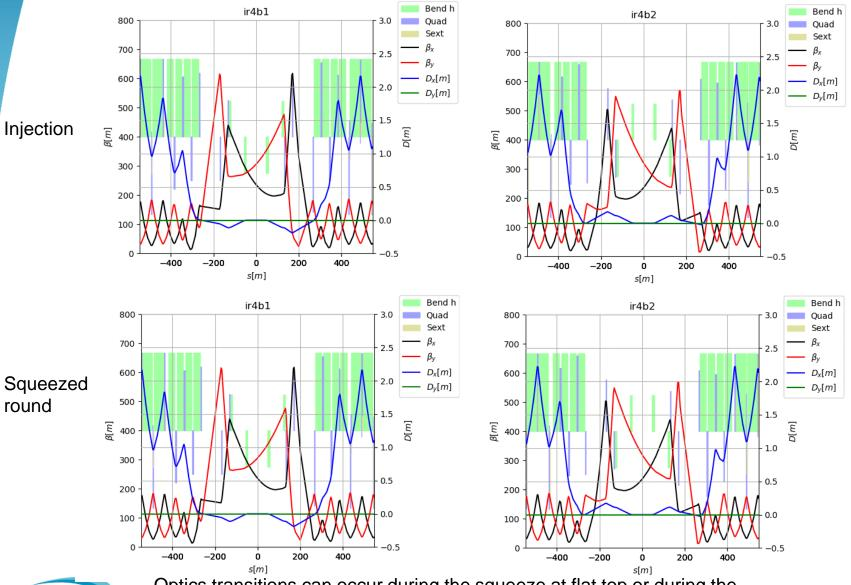
Optics transitions can occur during the squeeze at flat top or during the ramp&squeeze depending on the operational scenario.
