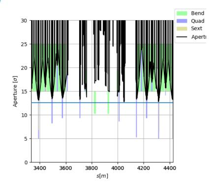
Aperture at injection above the target of 12.6  $\sigma$  using HL-LHC aperture tolerances.
