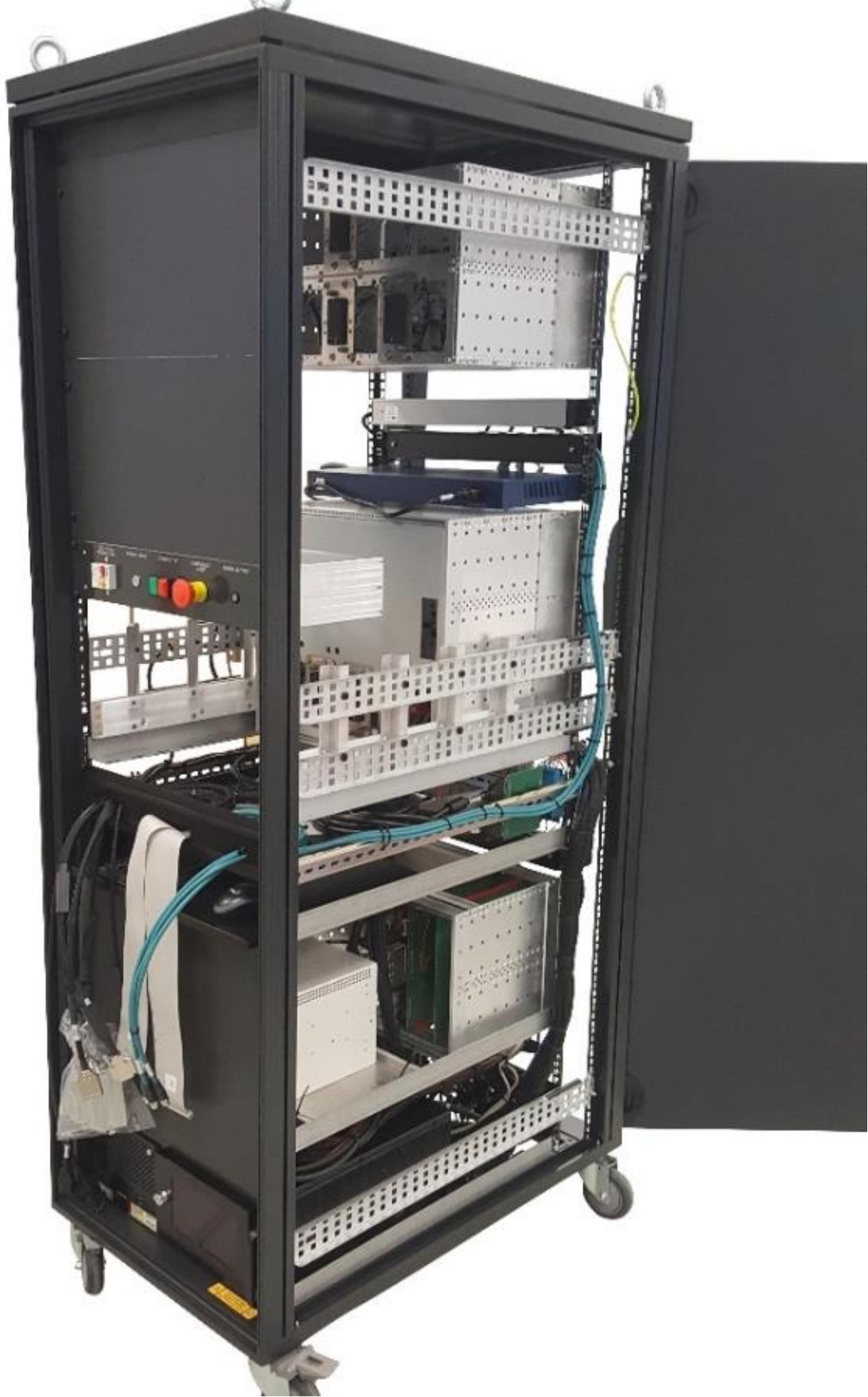
T&M / Satellites test bench, T&M rack integration
