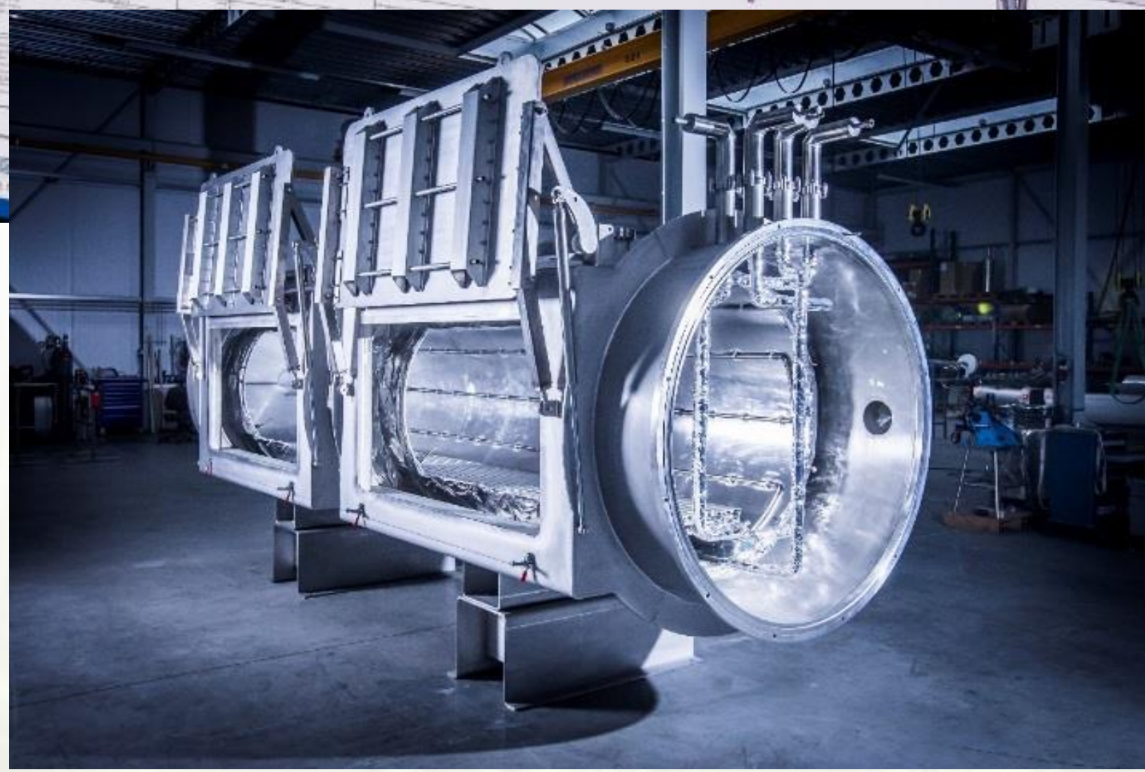
Universal testing cryostat GSI
