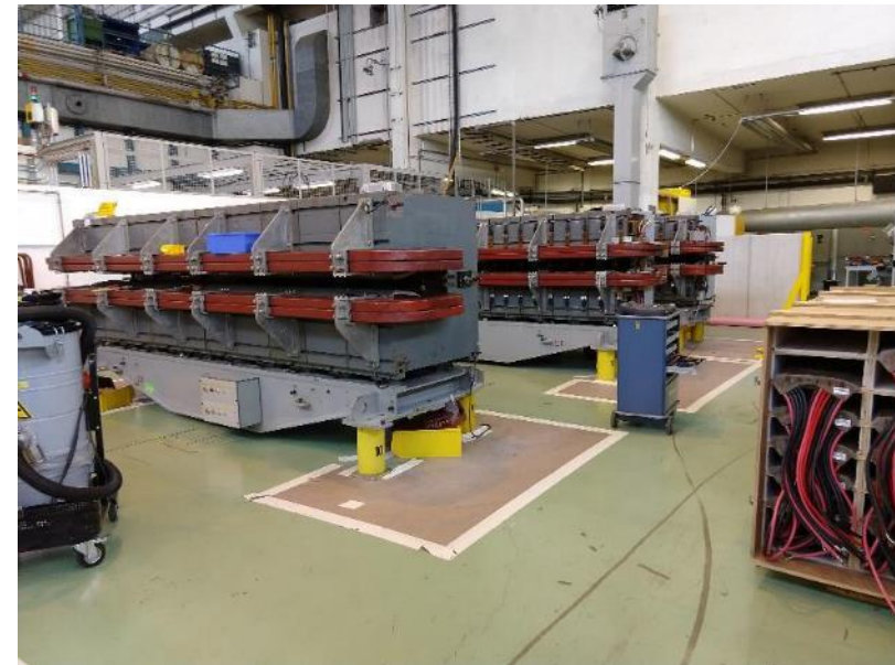
43 magnets (101 main magnets in PS)
