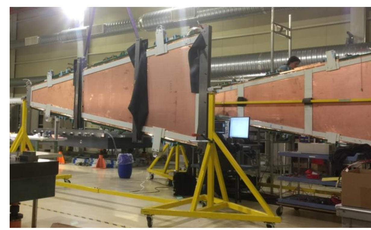
Assembled sTGC wedges, waiting for services and electronics
