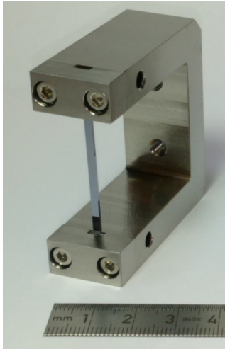
Si crystal is 0.8 mm wide, 2 mm long, 35 mm high
