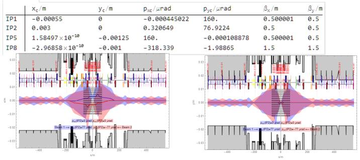
Horizontal parallel separation increased to ±3 mm IP shift bump still off Transition through zero external bump to unfavourable polarity with respect to IP (neutrons moving down) No sign of beam-beam effects.
