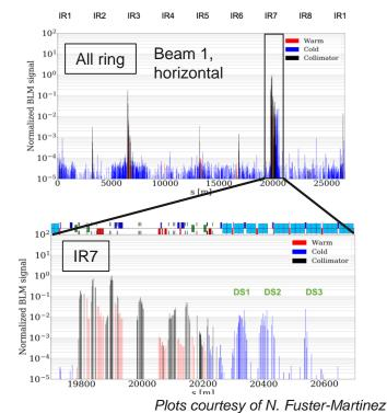
Measurement of collimation efficiency by introducing transverse losses on a safe low-intensity beam.
