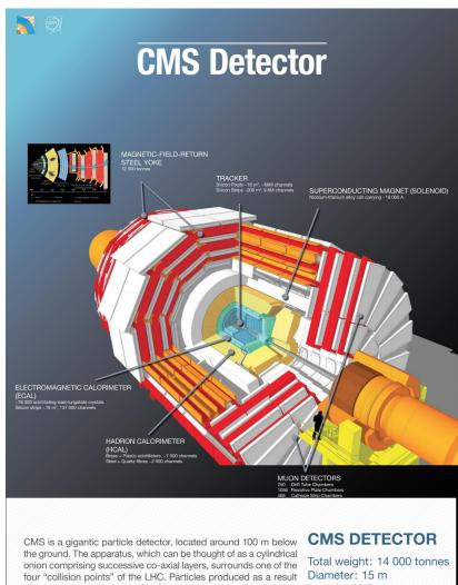
of proton-proton collisions fly through these layers, leaving their Length: 28.7 m traces in different CMS sub-detectors.
