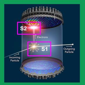
Two-phase Xenon TPC experiment for direct Dark Matter (DM) detection (<u>technical design report</u>)
