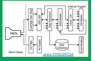
Full signal chain (PMT response, trigger logic)
