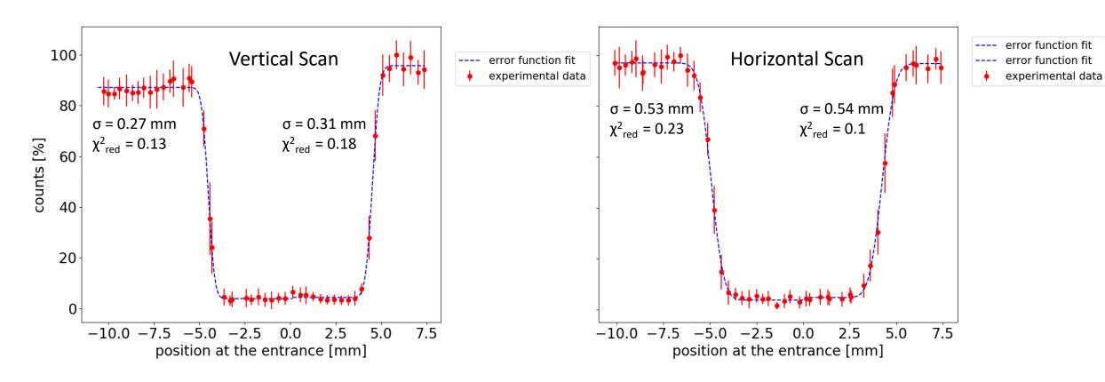
Effect of magnetic field on electron beam trajectory calculated as the difference between the two scans (considering proton beam trajectory straight)
