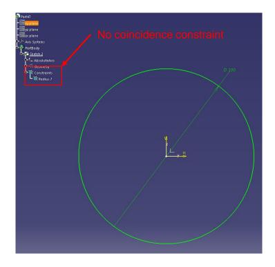
In this case the circle centre is fixed to the origin but no visible constraint exists
