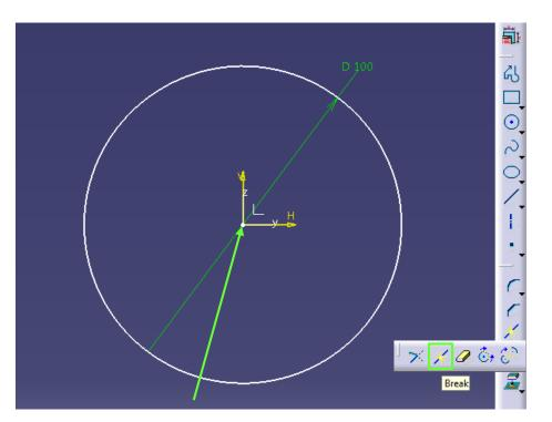
By using the Break function on the center point, it can be isolated
