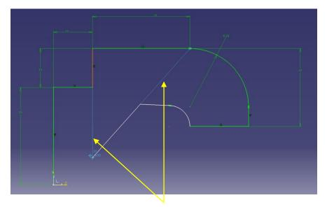
Automatic constraints detection and creation is often useful to design a shape But in some case it can lead to unwanted constraints creation or inconvenience during manipulation
