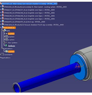
Create a new part which contains the cutting element. This element must be published
