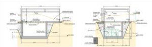
FIG. 41: Typical Sections through the experimental hall parallel to the beam-line (left) and transverse to the beam-line (right)
