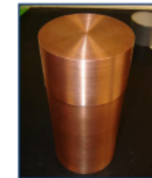
Housing made at LSC of electroformed copper
