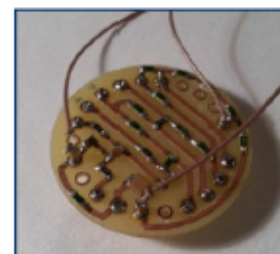
Voltage dividers in cuflon PCB
