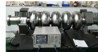
CEPC 650 MHz 5-cell cavity with waveguide HOM coupler by HERT
