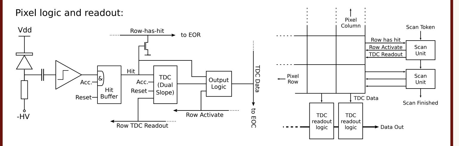
• Measures the timing of an instantaneous burst of many photons • Application: ToF camera, LIDAR, fluorescence lifetime imagine
