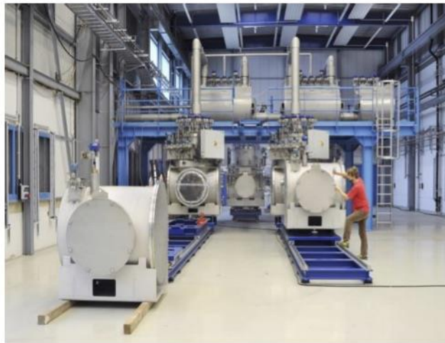
GSI: Series test facility for the SIS100 s.c. dipole magnets, string test, current leads and local cryogenics components.
