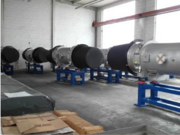
41 sc dipole SIS100 modules manufactured at BNG and shipped to GSI. 36 accepted
