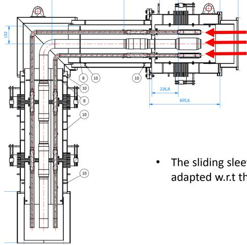
Each process pipe has been "pushed" by  $\approx$  20 mm to allow the thermal shrinkage at cold without residual stress
