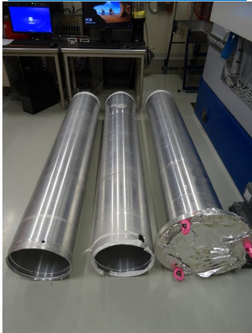
Low dose upper part of the beam pipe (3 x 2 m, 1 x 1.2m)
