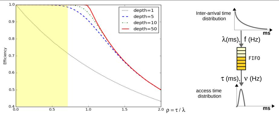
• Efficiency vs traffic intensity ( $\rho = \tau / \lambda$ ) for different queue depths
