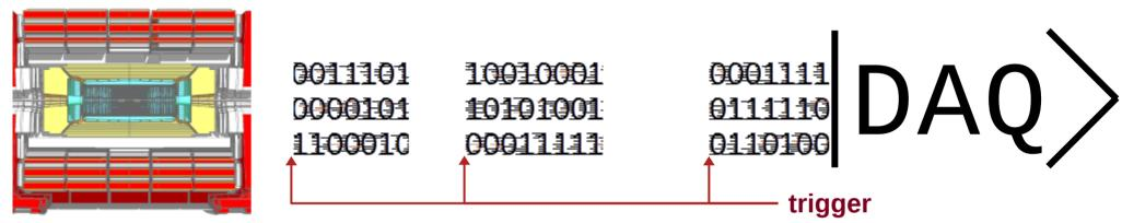
• **Triggerless**: the detector push data at its speed and the downstream daq must keep the pace
