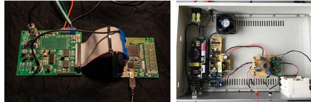
Working prototypes of signal generator and modulator
