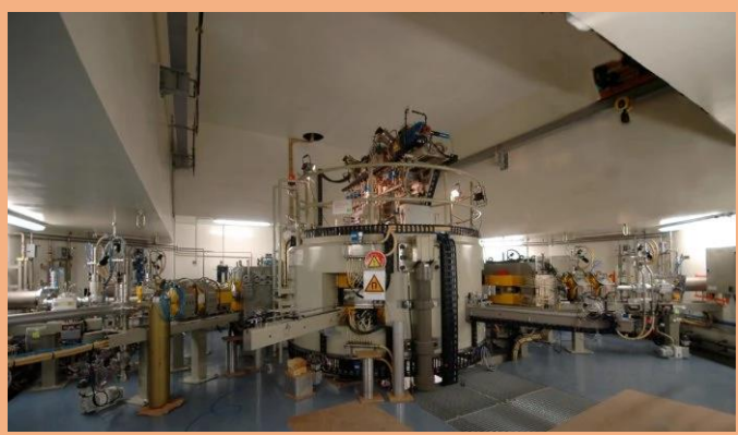
Cyclotron C70 – Nantes, Fr Protons between 30-70 MeV
