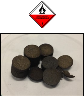
Uranium carbide pellets d=14 mm Thickness 1.5 mm
