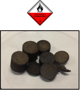
Uranium carbide pellets d=14 mm Thickness 1.5 mm
