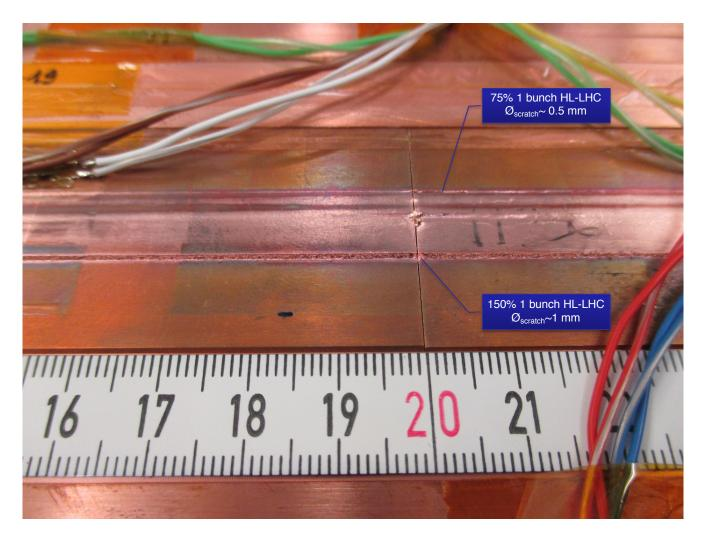
Small surface stripe for the case tested with 75% of 1 HL-LHC bunch (Cu layer removed for 150% of the HL-LHC bunch)
