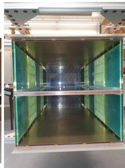
Two anodes, installed inside field cage
