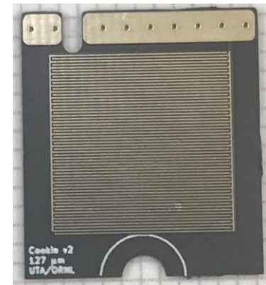
127 \mu\text{m} trace spacing 5V/ \mu\text{m} max field UTA/ORNL
